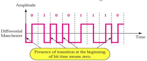
In differential Manchester encoding, the transition at the middle of the bit is used only for synchronization. The bit representation is defined by the inversion or noninversion at the beginning of the bit. **IEEE802.11: Frequency Hopping (FHSS) and Direct Sequence (DSSS):**
