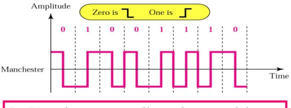
In Manchester encoding, the transition at the middle of the bit is used for both synchronization and bit representation.
